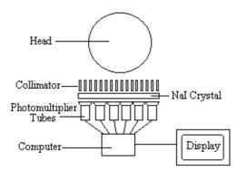
Figure 3.1 Schematic diagram of a gamma camera used in SPECT imaging
