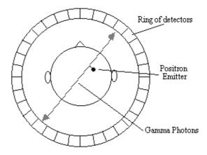
*Figure 3.2* Schematic diagram of a PET scanner. A positron is emitted from a radioisotope in the brain. The positron annihilates with an electron, producing two photons emitted at 180 degrees to each other
